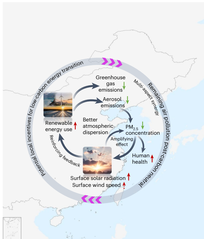
Fig. 5 | Conceptual model of multi-aspect synergies and renewable self-reinforcing effects. Grey arrows indicate the linkages between renewables penetration, air quality, greenhouse gas emissions and renewable energy performance, primarily in eastern China. Red and green arrows show respective increase and decrease of each parameter. Dashed red arrows indicate generally weaker wind speed increases in comparison to solar radiation. Grey rings indicate the self-reinforcing renewables may provide additional incentives for post-carbon neutral renewable energy promotion to address the remaining air pollution, together with other air pollution mitigation practices (for example, efficiency improvement and emissions mitigation from industrial processes). Chinese map from the Resource and Environment Science and Data Center, Institute of Geographic Sciences and Natural Resources Research, Chinese Academy of Sciences ( https://doi.org/10.12078/2023010103 ) 37 . World map underneath sourced from Natural Earth ( https://www.naturalearthdata.com/ ).
